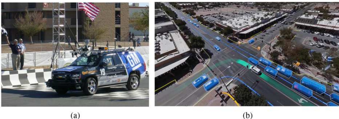
(a) Autonomous car Boss which won the DARPA Urban Challenge. Photo by Tangi Quemener/AFP/Getty Images/Newscom. Courtesy of Sebastian Thrun. (b) Aerial view showing the perception and predictions of the Waymo autonomous car (white vehicle with green track). Other vehicles (blue boxes) and pedestrians (orange boxes) are shown with anticipated trajectories. Road/sidewalk boundaries are in yellow. Photo courtesy of Waymo.
